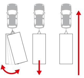
The driving behaviour of the trailer is permanently monitored by the ATC. Sensors detect dangerous lateral movements directly
