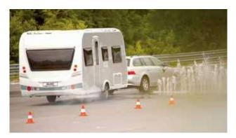
The AL-KO ATC stabilisation system can be operated in addition to trailer ESP in the car, such as is offered by some car manufacturers.
