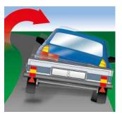
The test vehicle combination with an unbraked trailer loses traction during emergency braking on a corner, skids and cannot be controlled.
